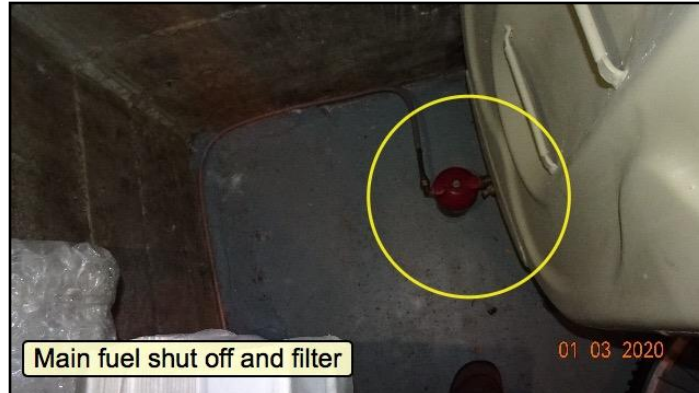
24. Main fuel shut off
